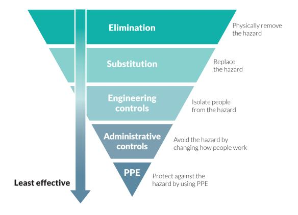
Figure 23.2. The hierarchy of hazard controls
